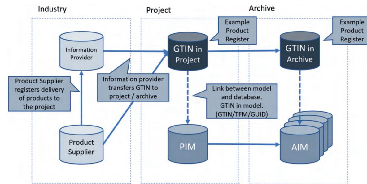
Fig. B1 - GTIN is in the building owner's product register. (PIM = Project information model, AIM = Byggverket's information model, operation)
