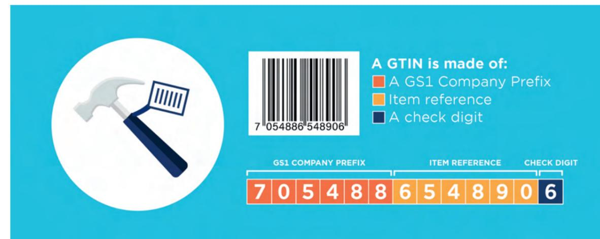
Fig. 6.1 Example of structure of GTIN-13 with 6-digit GS1 Company Prefix
