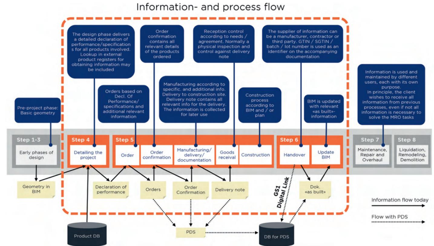
Fig. 7.1 Fig 7.2 Model for generic information and process flow
